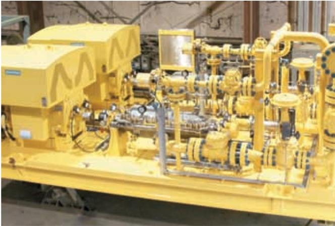
By bringing in 2 MW of Rental Power from Cummins Power Generation, IFS engineers tested all phases of the pumping system at full capacity prior to its installation.
