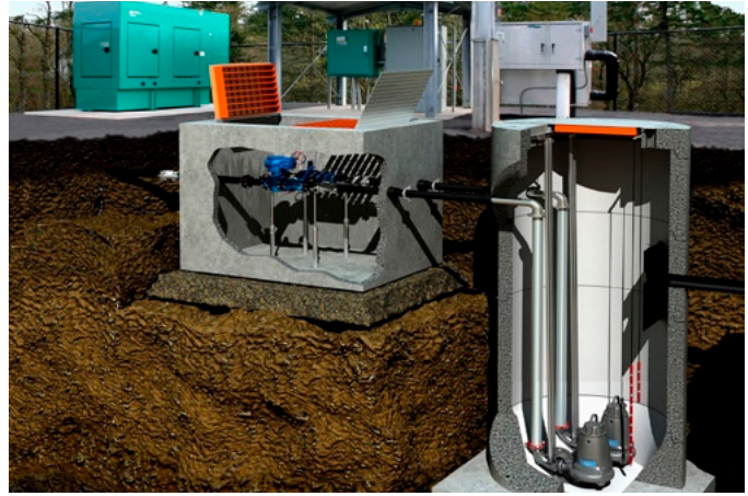
Pre-engineered sewage lift stations include submersible pumps, an underground valve vault, a standby generator and controls.
