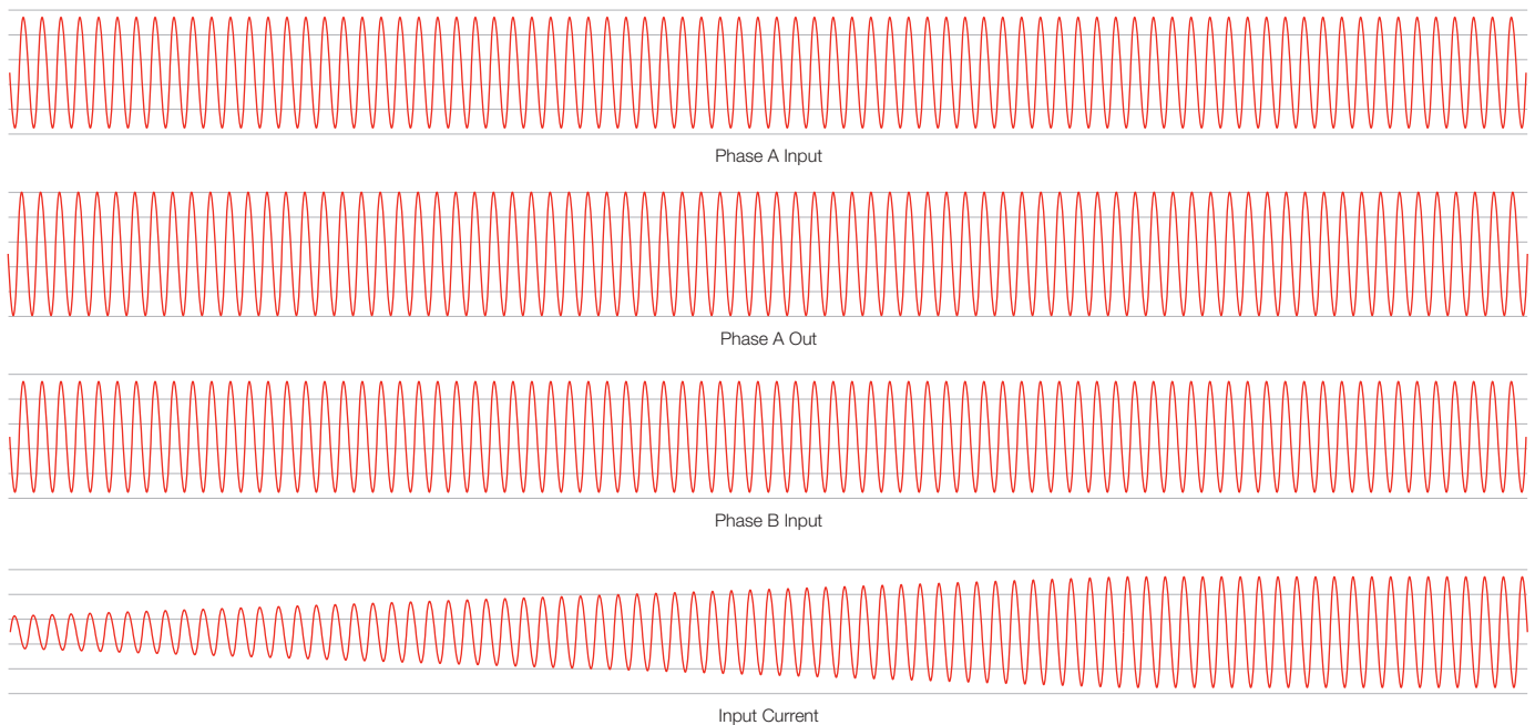
FIGURE 6a – The top recording is an A-phase voltage. The second recording is an A-phase output current from UPS. The third recording is a B-phase input voltage to UPS, and fourth line is an input amperage to UPS rectifier.
